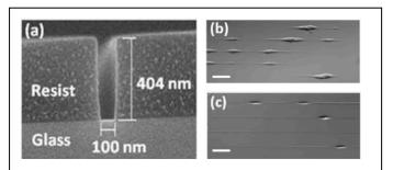
Fig. 1. (a) SEM image of cross section of the EB lithographed nano line pattern. (b,c) hbmMSC cultured on the line patterns of 500 nm width. (b) 100 nm depth and (c) 400 nm depth. Scale bar =100  $\mu$ m.
